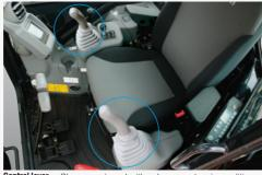
ontrol lever Shown equipped with cab, armrests, air conditioned pedal and FM/AM radio as optional items.
