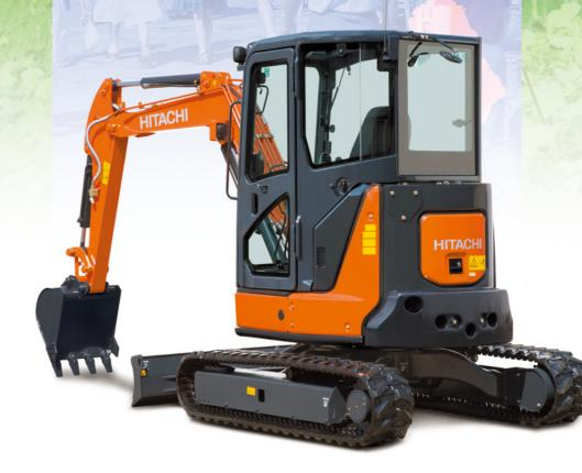
Shown equipped with 1.52 m arm, additional counterweight, cab and extra piping and as optional items.
