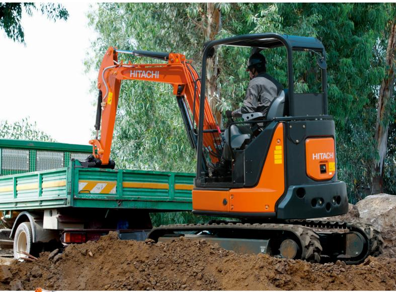
Shown equipped with 1.52 m arm, additional counterweight, armrest and extra piping as optional items.
