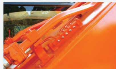
Centralized boom and arm greasing points
