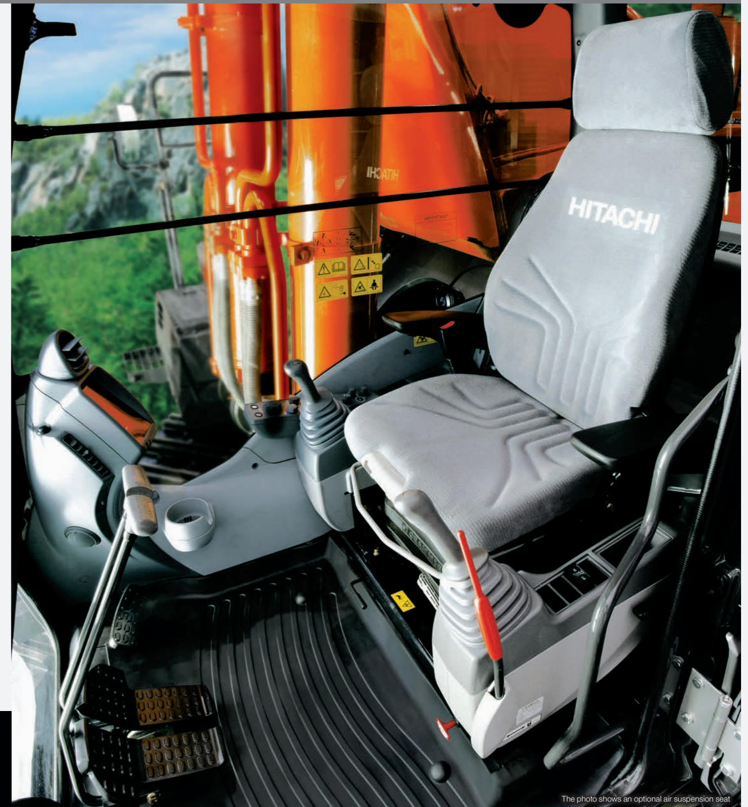
The photo shows an optional air suspension seat
